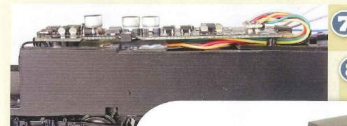
There may be enough dearance for the decoder to fit above the PCB, but there are a number of components which might interfere. I decided to locate the decoder below the PCB and between the
