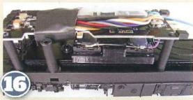
The speaker was fitted to the ballast weight on the floor of the chassis and the decoder end was wrapped with black tape to secure it in position and to disguise the view of the wires through the exhaust ports - not obvious until the body has been refitted.
