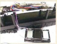
The purple speaker wires from the decoder were connected to the speaker next preparing the speaker endosure for final installation.
