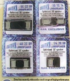
Zimo has recently released a small range of high performance speakers designed to make it easier to install quality speakers in a low profile environment. From these I have selected the LS40x22x09 twin driver 3D speaker for the HST project.
